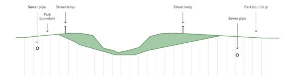
**Figure 5.12:** Cross-section profile showing earthworks excavation for the grey infrastructure solution. Green shading indicates the extent of excavation.
